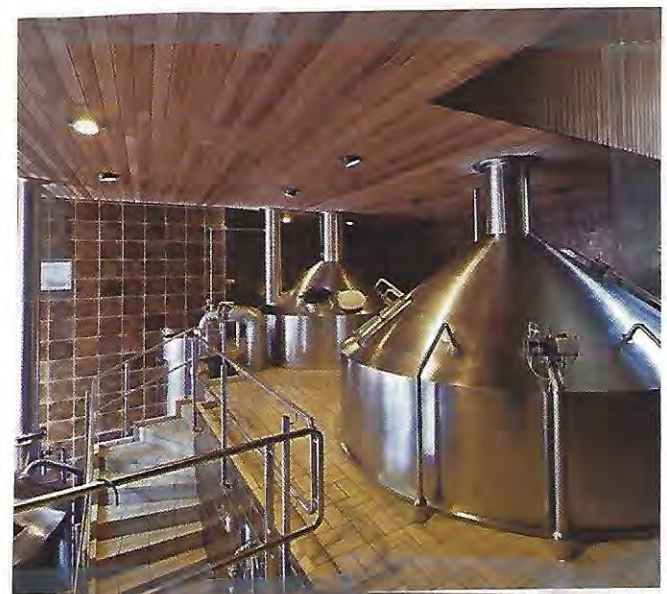
THE MASH TUNS ARE WHERE THE BREWING PROCESS BEGINS.
